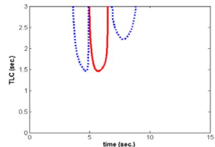
Fig. 7.: Time to Line Crossing, reference case (left: solid, right: dotted)
