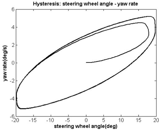
Fig. 4.: Steering wheel angle – Yaw rate hysteresis curves at 1 Hz
