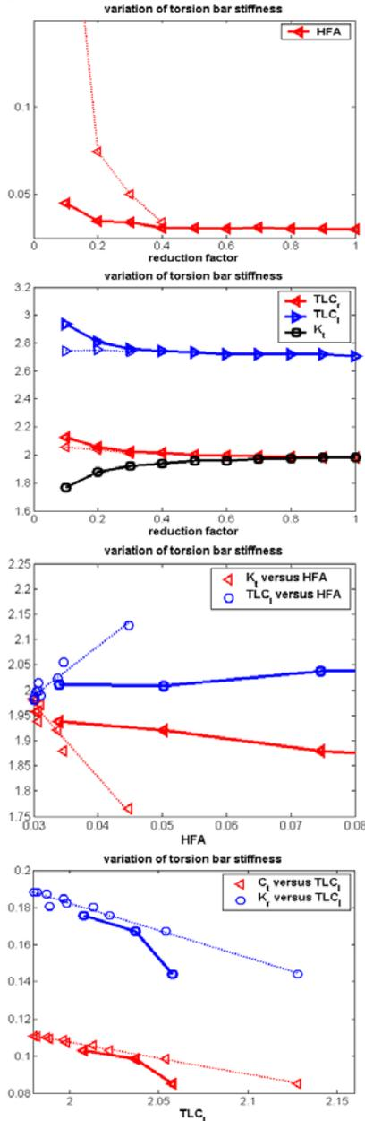
Fig. 8.: Variation of workload-, steering performance- and steer feel indicators for a single lane change, varying torsion bar stiffness
