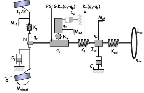
Fig. 1.: Model of the steering system
