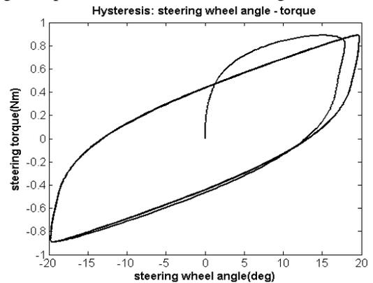
Fig. 3.: Steering wheel angle - Steering torque hysteresis curves at 1 Hz
