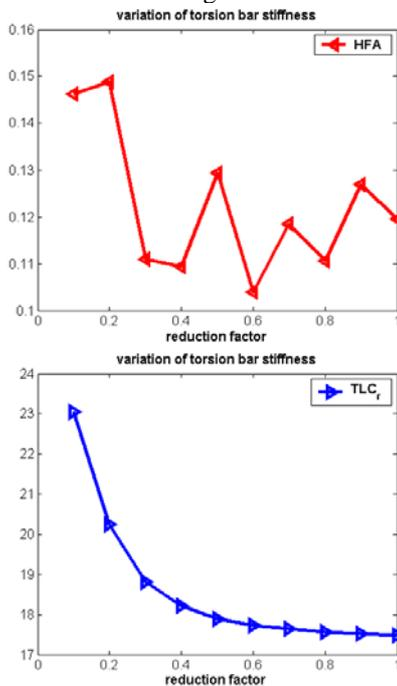
Fig. 10.: Variation of HFA and TLC for a single u-turn, varying torsion bar stiffness
