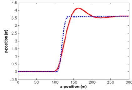
Fig. 5.: Lane change trajectory (dotted) and vehicle path, (solid)
