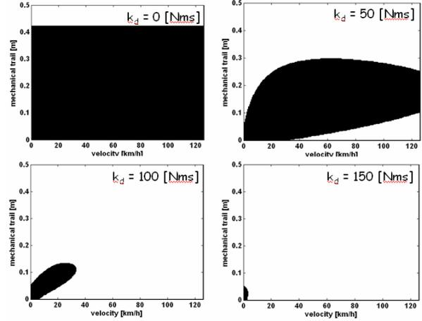
Fig. 10.: Areas of instability for the wheel system of fig. 9.
