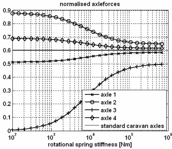
Fig. 5.: Normalised axle forces under steady state conditions, for varying rotational spring stiffness, linearised model.
