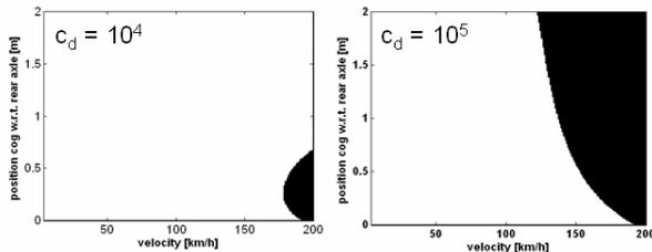
Fig. 12.: Areas of instability of different values of  $c_d$ .
