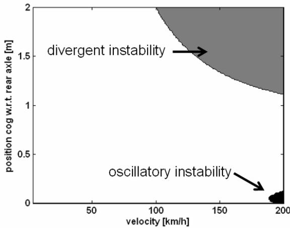
Fig. 11.: Areas of instability for the vehicle-caravan system
