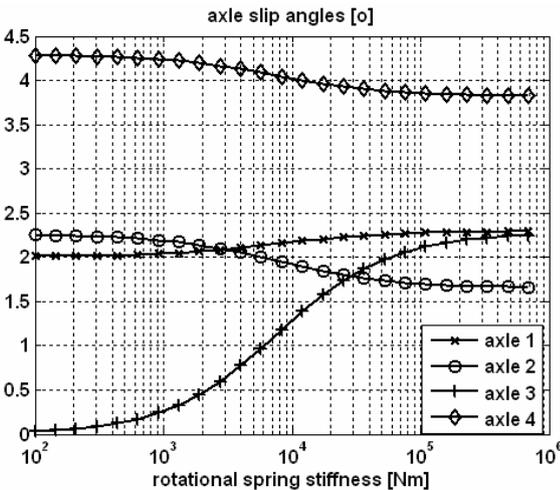
Fig. 6.: Axle slip angles for varying rotational spring stiffness, linearised model
