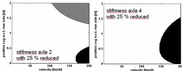
Fig. 13.: Areas of instability for adjusted axle stiffnesses,  $c_d = 10^4$  Nm
