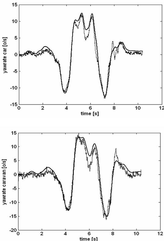
Fig. 4.: Yaw rate results, simulation vs. experiments.
